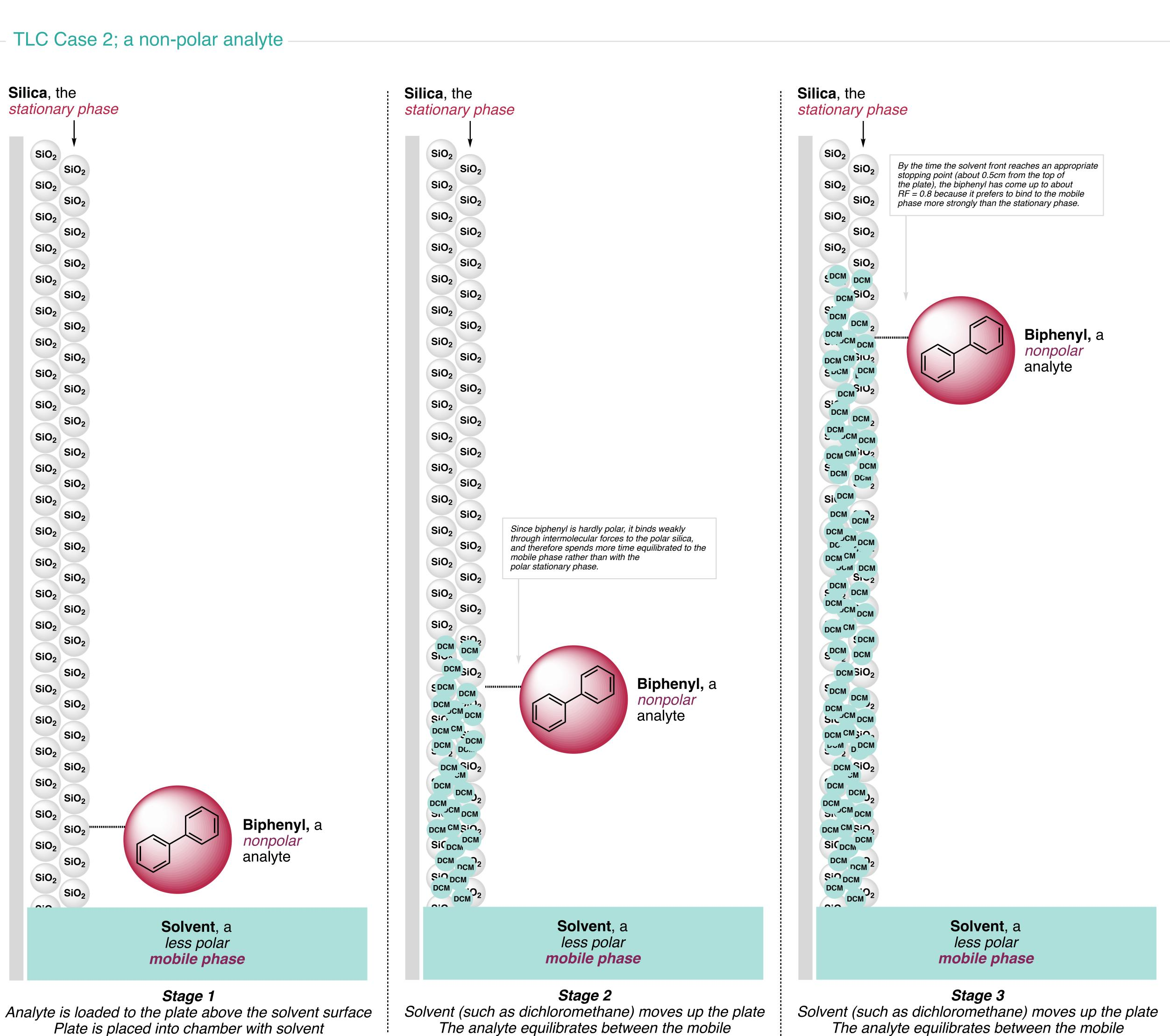
(solvent) and stationary (silica) phases
